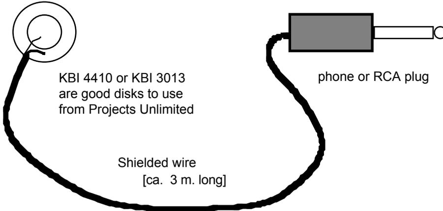
NOTE: if you make this wire longer than it needs to be, there will be less stress on this solder connection, which is weaker than the other
